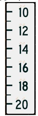
Figure 11. Drawing of what a vertical gauge board looks like. It would be in the water, and the waterline would cross a number and would provide the actual realtime vertical clearance at that bridge or overhead obstruction.
