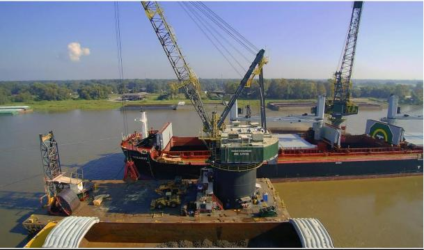
Figure 3. Photograph of the Crane Barge MR ERVIN. The photograph depicts the barge in operation working a ship moored to a midstream facility in the Mississippi River. Note also the Crane Barge HULK on the far side of the ship in the background of the picture; provided by Cooper Consolidated.
